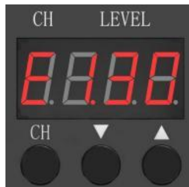
Figure 5: Millisecond Strobe Timing Setting
