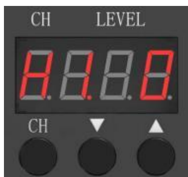
Figure 2: Normally-Off Mode Setting
