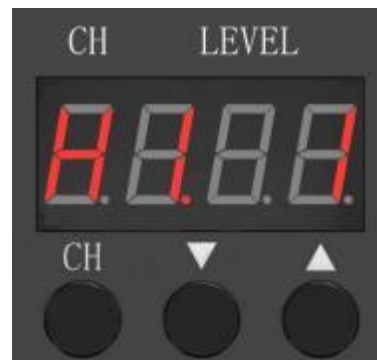
Figure 3: Normally-On Mode Setting
